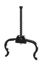
There's no pre-installation necessary—attach the clip's legs onto the joist, slide the clip into the groove, place the adjacent board, and drive the fastener into place. I was impressed with how securely they grasped onto the joist, making it easy to keep going and not pause for adjustments.
